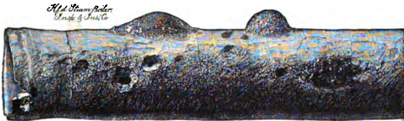
FIG. 16.—Tube Pitted by Pure Water.
